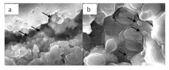
Figure 2. The scanning electron microscope images of *Acetobacter aceti* biofilm on screen printed carbon electrode. (a) before measurement and stored for 17 days, (b) after repeated measurements and stored for 17 days, observed at 10,000 magnification
